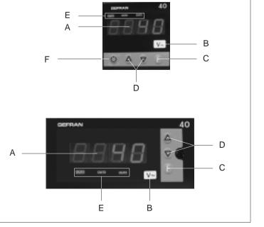
Red LED display IP65 faceplate protection *WEIGHT* 160g. (48 format), 320g. (96 format) in the complete version
